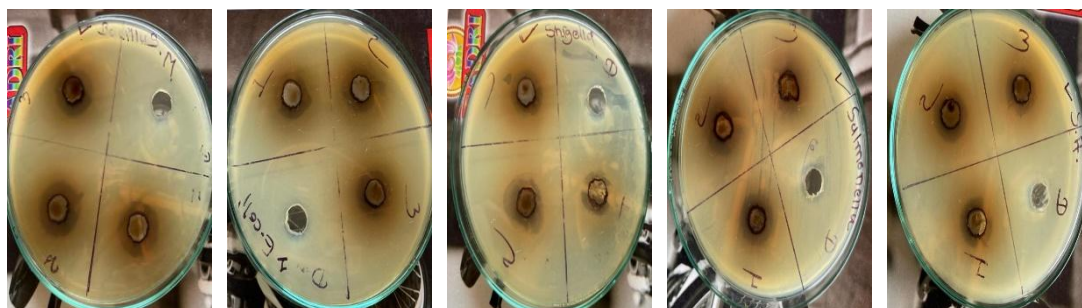
Fig. 2: Zone of inhibition of Piper longum plant extract against Escherichia coli , Bacillus megaterium , Shigella flexneri , Salmonella enterica typhimurium , and Staphylococcus aureus respectively.
